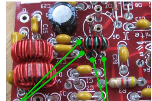
Connect secondary leads, to two S pads at ends of C14 and C17 pads
